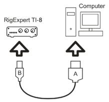
Once the cable is connected, computer detects a new device. The user does not have to interact at this step.
