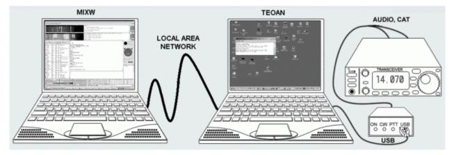
Left side: computer (network name: **dn-acer**) running MixW software Right side: computer (network name: **dn-compaq**) with MixW RigExpert connected.
