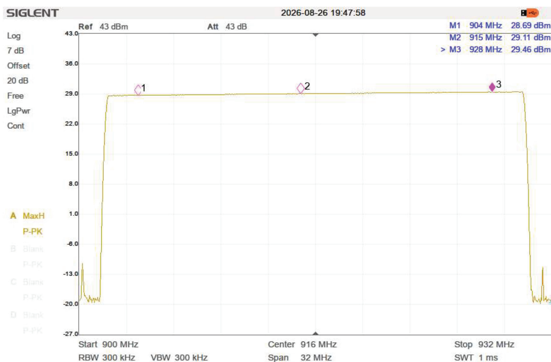
Figure 2. PA output power. Input RF signal CW 8dBm
