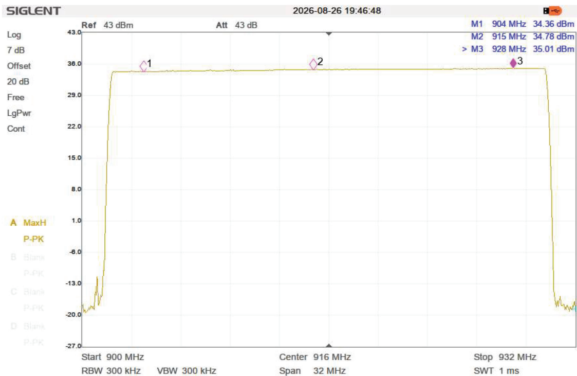
Figure 3. PA output power. Input RF signal Pulse 15dBm
